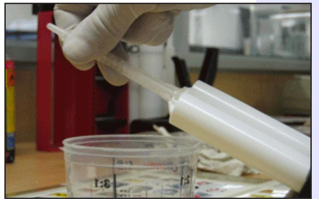
8 Now attach the static mixer to the cartridge. (This screws in)
