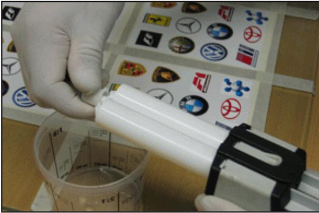
5 Remove safety cap from the cartridge by turning 90° and gently pulling
