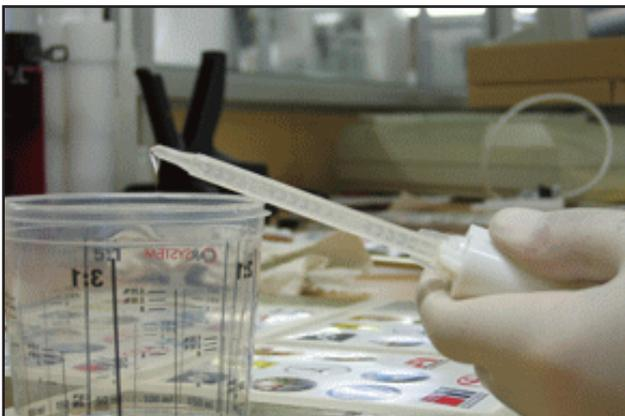
9 Pull gently on the trigger until resin is ejected from the end of the static mixer.
